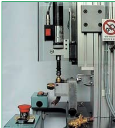
Workstation for the tightening/un-tightening of industrial valves
